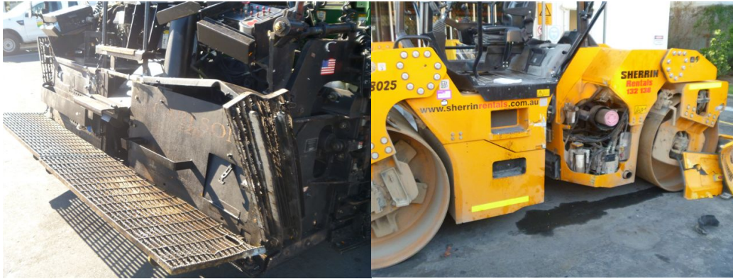
Damage to Paver rear right hand side
