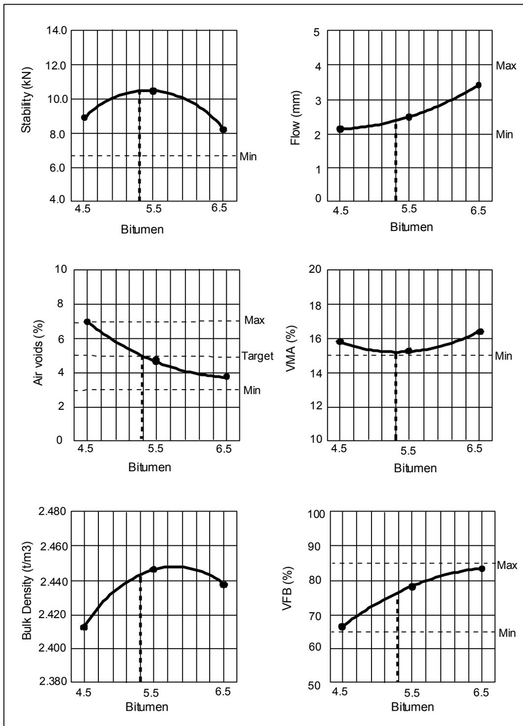
Figure 6 Marshall Test Results
