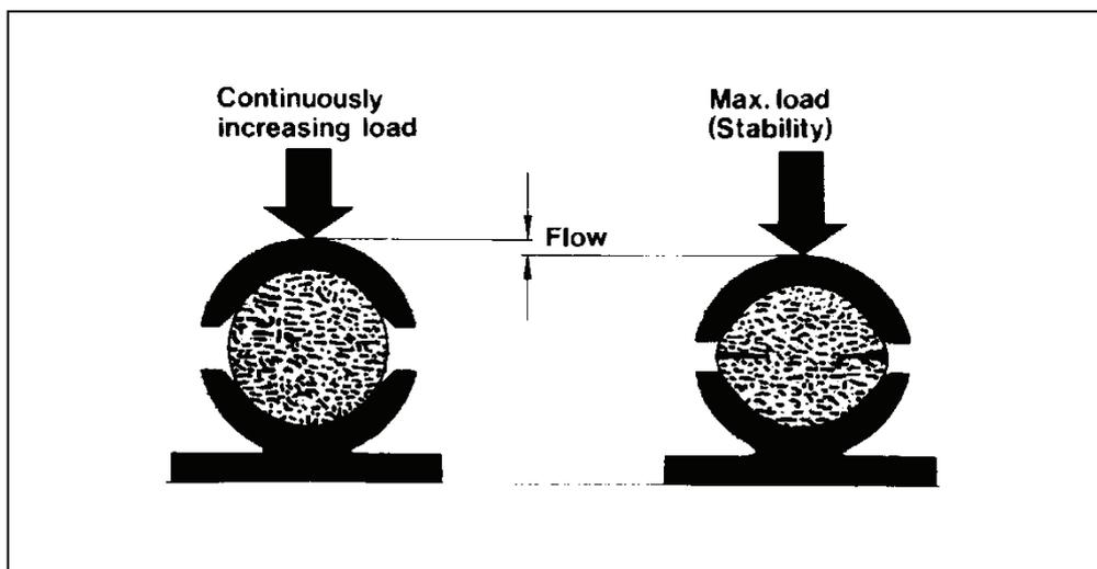
Figure 5 Testing of Marshall Specimen
