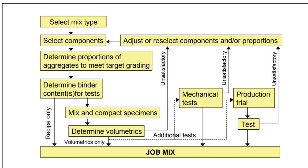
Figure 1 Asphalt mix design process
