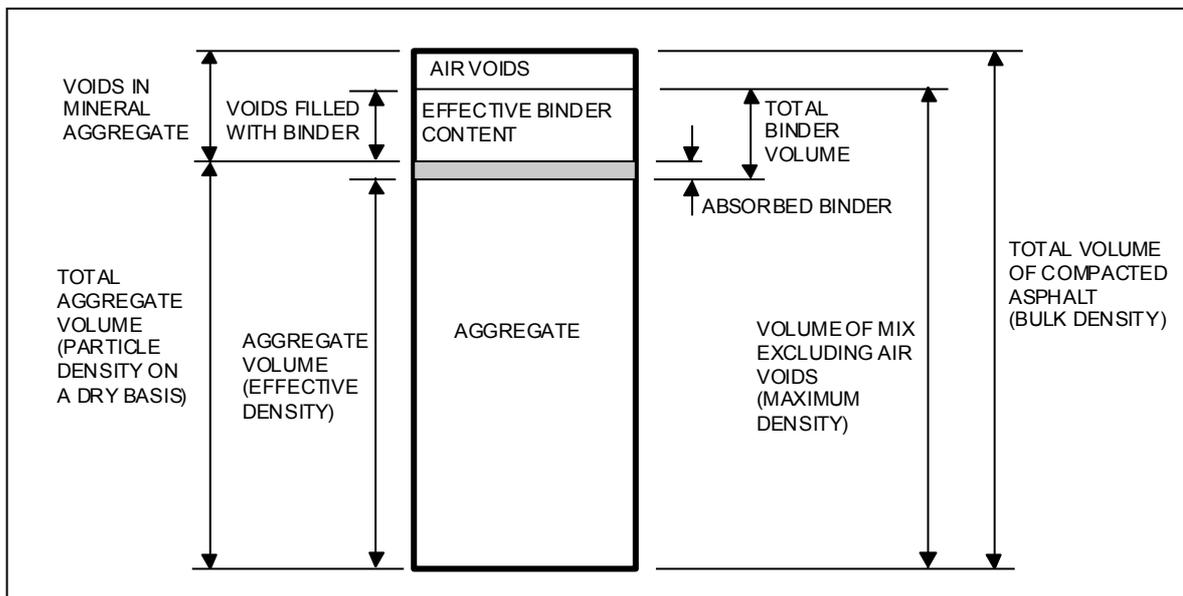
**Figure 2 Constituents of a Compacted Dense Graded Asphalt Mix**
