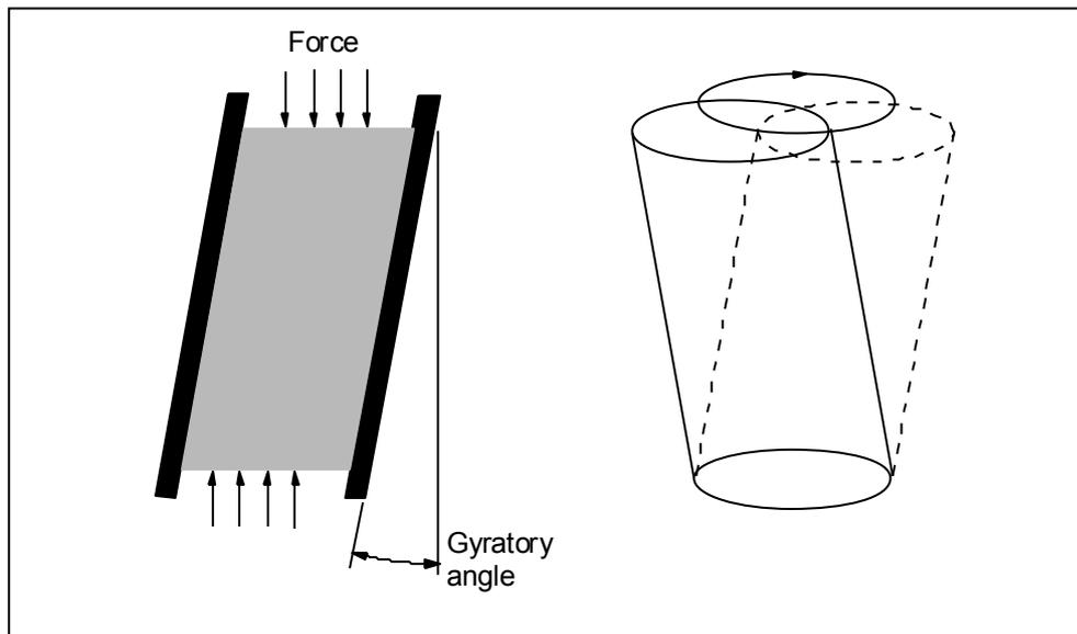
**Figure 4 Principle of Gyratory Compaction**
