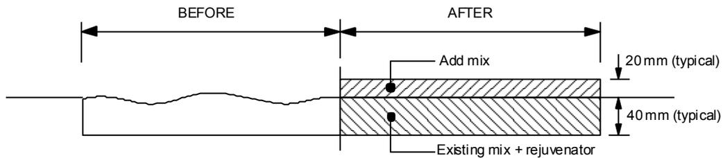
Figure 2 Repave procedure
