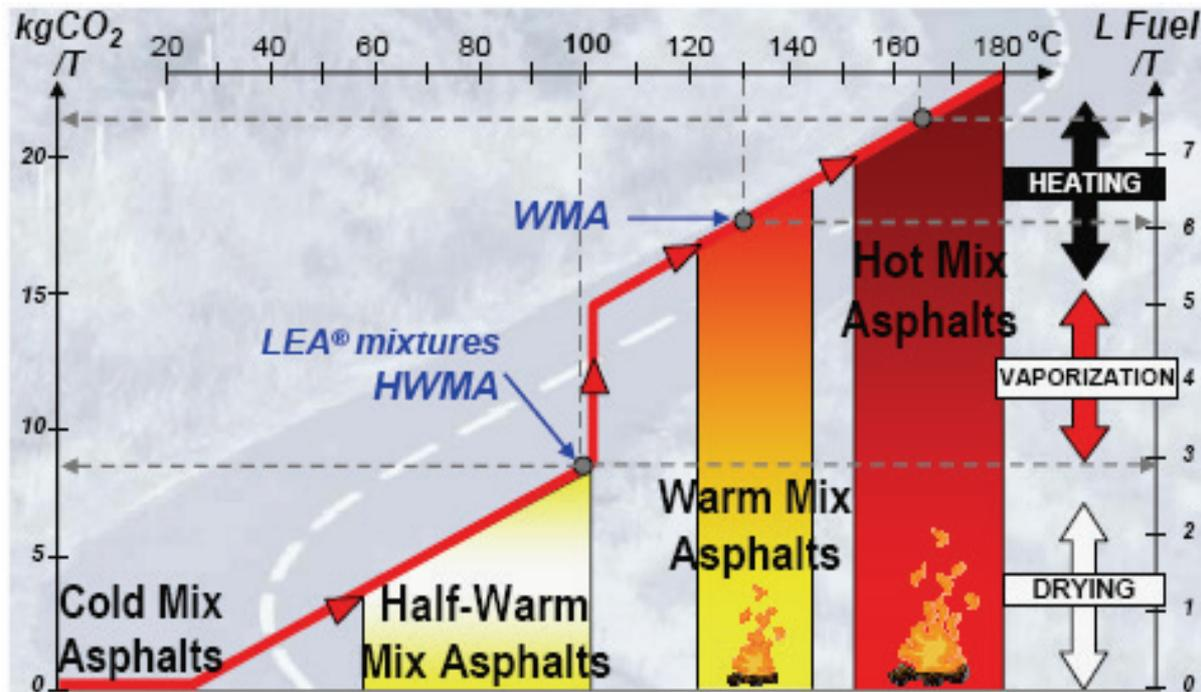
Figure 1: Classification by temperature range (Temperatures and fuel usage are approximations)
