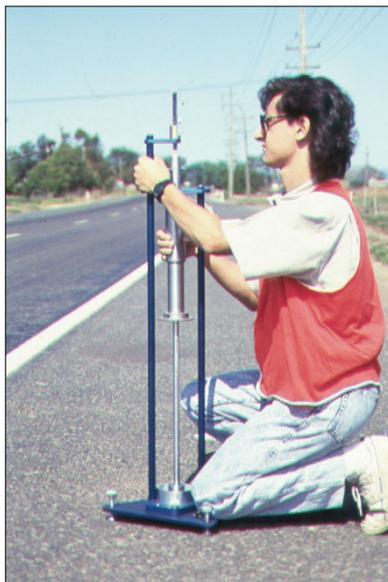
*Figure 18: Ball embedment testing*
