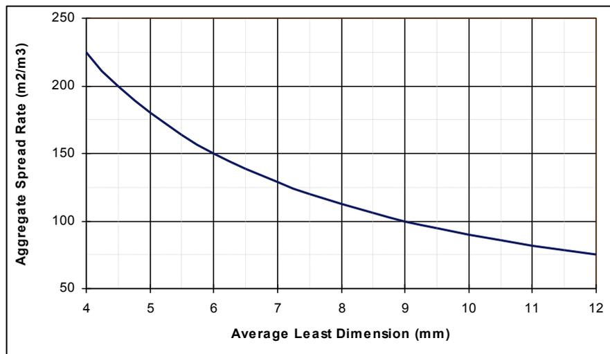
Figure 19: Loose aggregate spread rate for single/single seals
