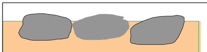
*Figure 17: Embedment of aggregate particles*
