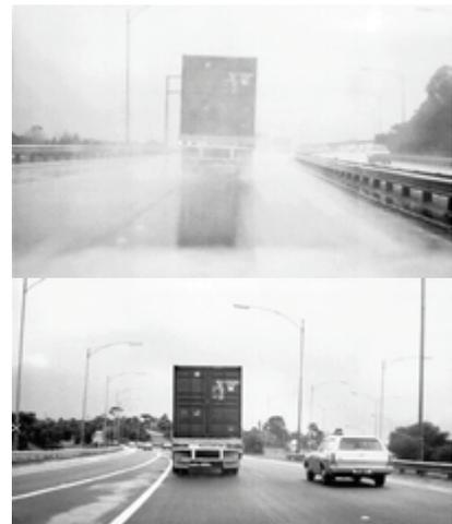
The above photos were taken within a short time of each other. The top photo shows a smooth surface with significant water spray. The open graded surface on the lower photo shows no spray
